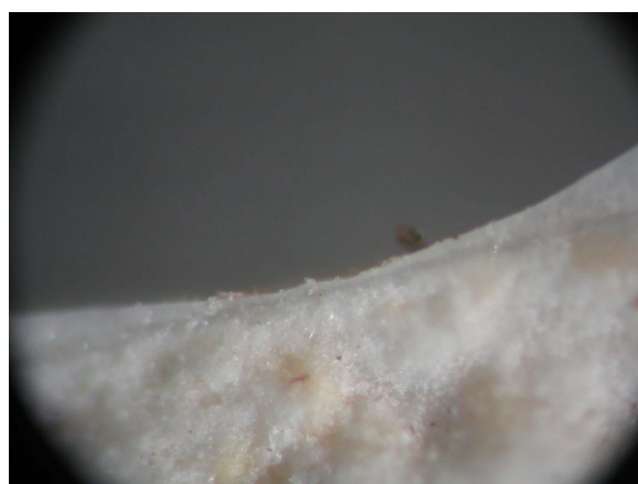
Fig. 3 Sectional view of the glaze contraction defect
